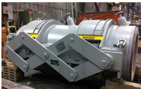
EagleBurgmann **high-end standpipe expansion joint** installed in a refinery in Texas, USA. Operating conditions:  $p = \dots 6.89 \text{ bar (100 PSI)}$ ;  $t = 510 \text{ }^\circ\text{C (950 }^\circ\text{F)}$ ;  $d = 1,170 \text{ mm (46")}$ . Medium: flue gas.
