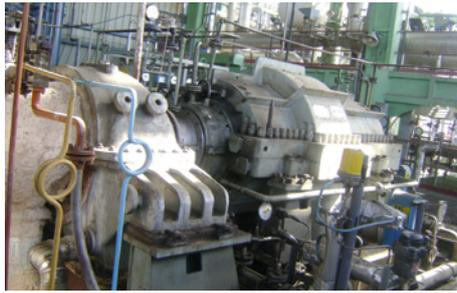
Bhel compressor in the delayed coker unit of the Panipat refinery run by the Indian Oil Corporation Ltd. The machine is equipped with EagleBurgmann **DGS20.1/200** tandem gas seals and a **diaphragm coupling**. Operating conditions:  $p = 6 \text{ barg (87 PSIG)}$ ;  $t = 150 \text{ }^\circ\text{C (302 }^\circ\text{F)}$ ;  $n = 8,909 \text{ min}^{-1}$ ;  $d1 = 180 \text{ mm (7.09")}$ . Medium: flue gas.
