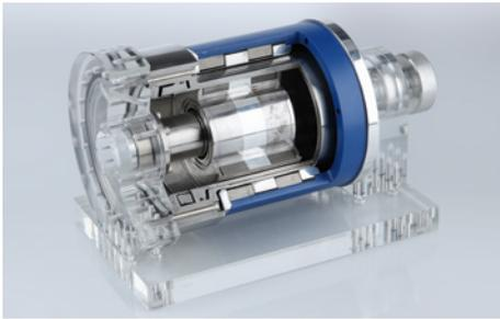
EagleBurgmann has designed a new high performance magnetic coupling type **NMB 22P-10R-65-ND2**. This is installed in a multistage vertical can pump of an ethylene cracker unit in a German refinery.  $p = \dots 65 \text{ bar (943 PSI)}$ ;  $t = -32 \dots +40 \text{ }^\circ\text{C (-26 }^\circ\text{F } \dots +104 \text{ }^\circ\text{F)}$ ;  $n = 2,980 \text{ min}^{-1}$ ; drive power: 315 kW direct start; design torque:  $>1,700 \text{ Nm}$ . Media: hydrocarbons C2+C4.
