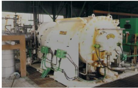
The hydro desulfurization unit of the refinery in Ciudad Madero, Tamaulipas, Mexico is equipped with a Mitsubishi compressor. It is reliably sealed by EagleBurgmann **SH6-D** dual mechanical seals. Operating conditions:  $p = 3.4 \dots 5.6 \text{ bar}$  (49 ... 81 PSI);  $t = 20 \text{ }^\circ\text{C} \dots 150 \text{ }^\circ\text{C}$  (68 °F ... 302 °F);  $n = 5,460 \dots 8,190 \text{ min}^{-1}$ ;  $d1 = 150 \text{ mm}$  (5.91"). Medium: gas.
