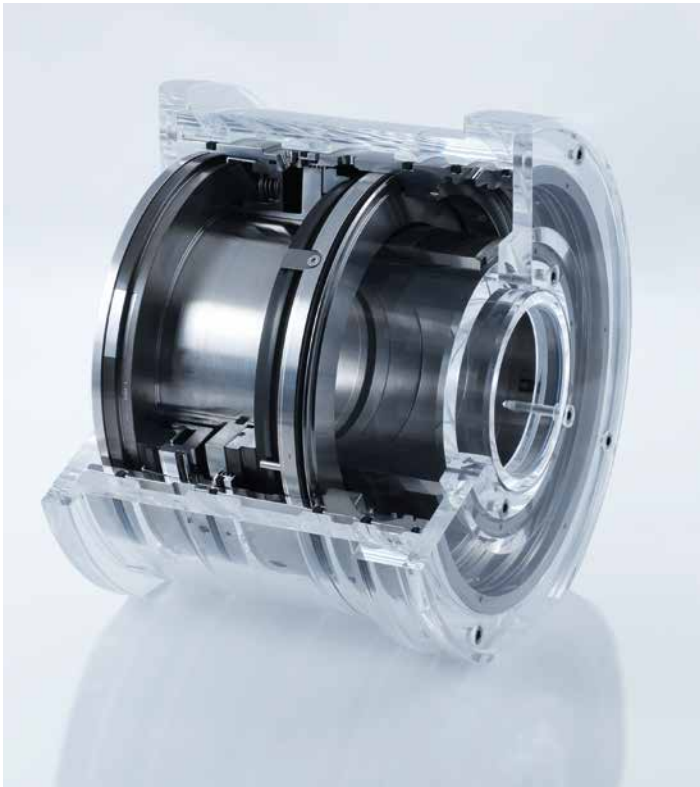
MDGS design example: Tandem seal with intermediate labyrinth. A typical solution used in combustible, toxic and environmentally harmful gases. The separation seal is an EagleBurgmann type CSE non-contacting carbon segment seal.
