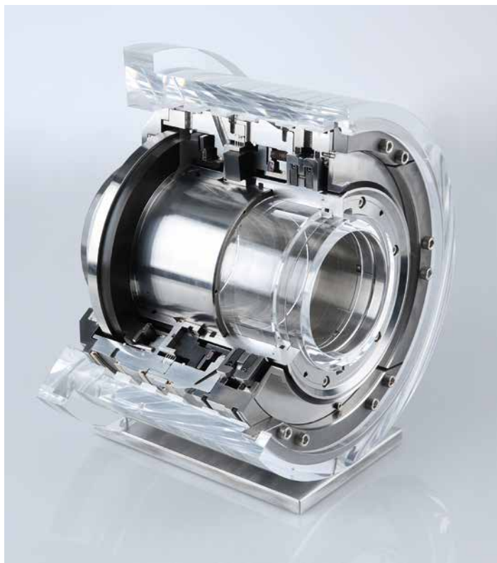
PDGS tandem seal with intermediate labyrinth and CSR separation seal for ultra-high pressure applications. This type is used, for example, in compressors for gas reinjection in offshore applications.
